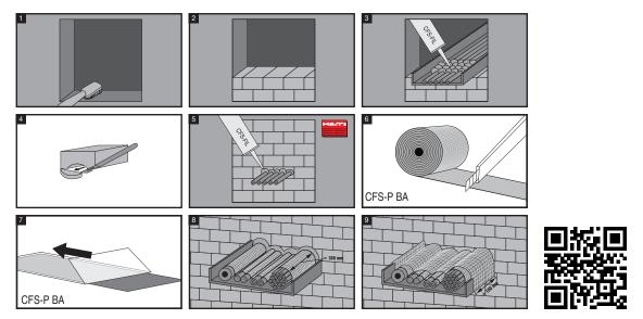
For some applications, firestop putty bandage CFS-P BA must be installed to upgrade the firestop classification to EI 120 (see pictures 6–9).
